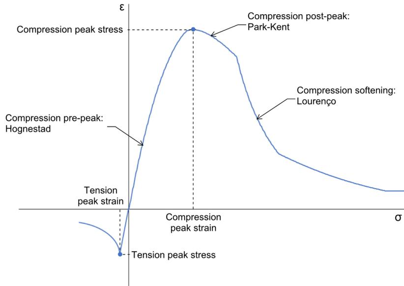
Figure 1. Masonry stress-strain curve
