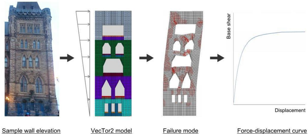
Figure 2. Procedure for determining force-displacement curve for a wall using the VecTor2 software suite
