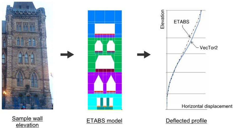
Figure 6. Procedure for determining wall stiffness using the VecTor2 software suite and ETABS
