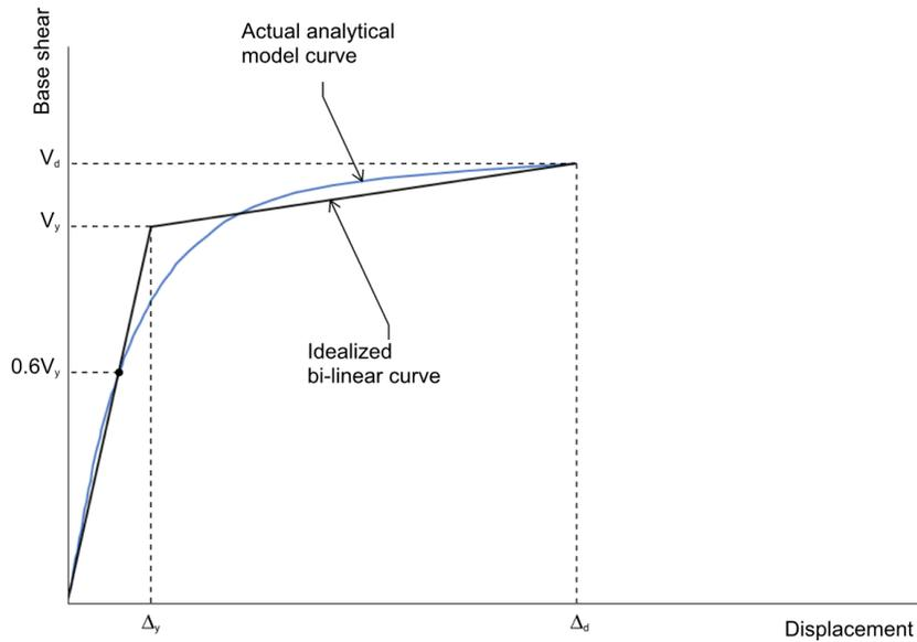
Figure 4. Analytical and idealized force-displacement curves for sample wall
