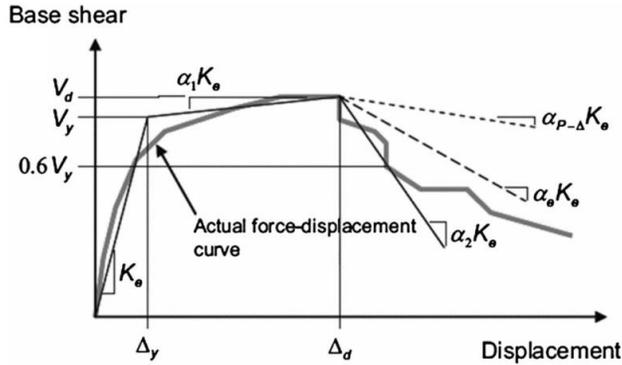
Figure 3. Idealized force-displacement curve [2]
